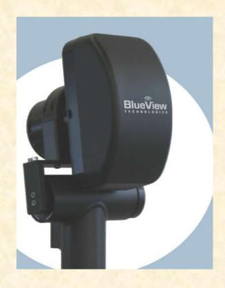
The BlueView BV5000 3-D mechanically scanning sonar head creates high resolution imagery of structures and objects and a 3-D point cloud that can be brought into CAD for modeling.
